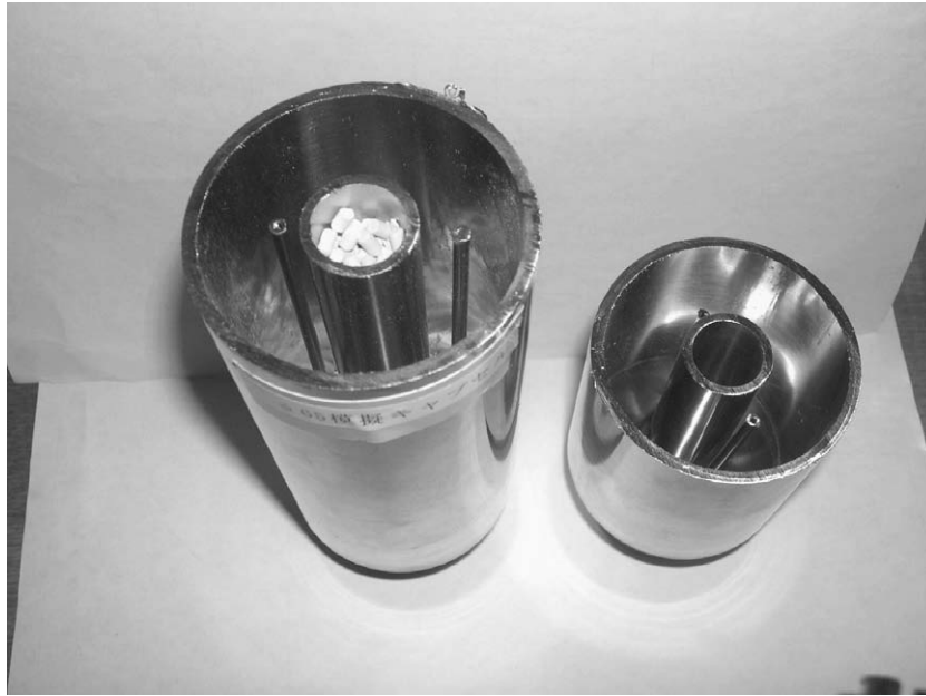
Fig. 3. Cross-section of a mockup of an irradiation capsule for tritium breeder materials. The mockup was cut in a test for trial fabrication of the dismantling apparatus.
